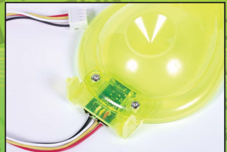
FIGURE 18. Install the IR sensors so that they face downward towards Binary Player Robot.
